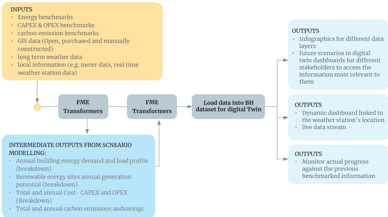
**Figure 12 Inputs and outputs in FME and Buro Happold Digital Twin**
