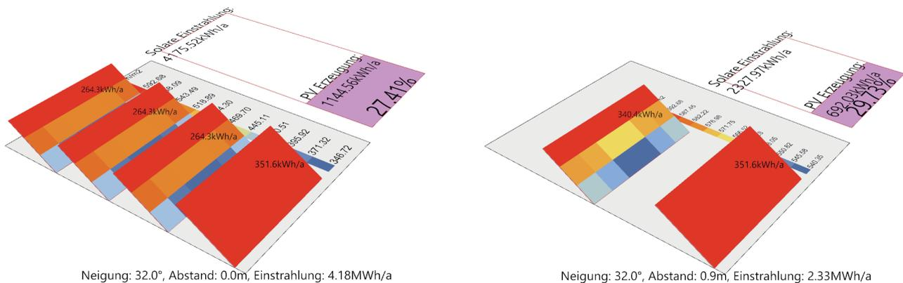
**Figure 6** Advanced method to calculate panel specific radiation and PV power in grasshopper , illustrated by authors
