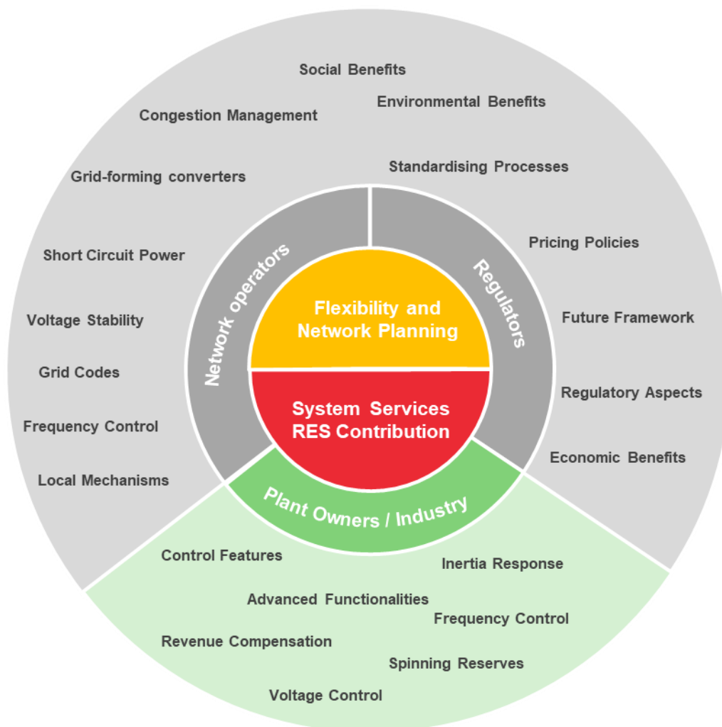
Figure 4-1: Summary of key points and topics that are related to the decentral provision of ancillary services
