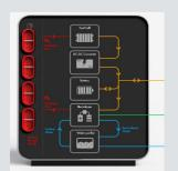
LAVO introduced integrated hybrid hydrogen batteries which combine rooftop solar and green hydrogen. The fuel cell is used to cover energy stored in the hydrogen back into electrical energy. The storage is able to cover an average household for two days.
